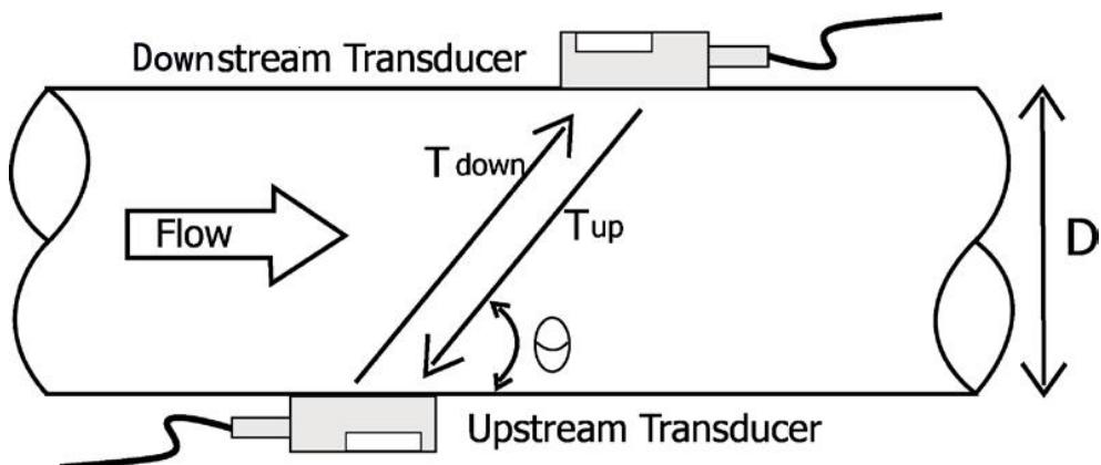
$$V = \frac{MD}{\sin 2\theta} \times \frac{\Delta T}{T_{up} \bullet T_{down}}$$
